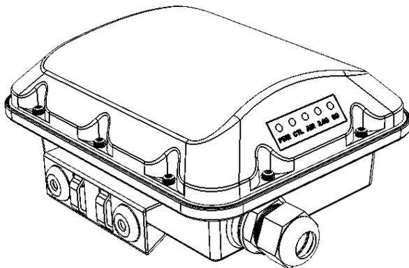
1. Feed the end of the cable through the sealing nut, rubber O-ring, clamping ring assembly, and cable gland base, as shown in [Figure 7](#).
